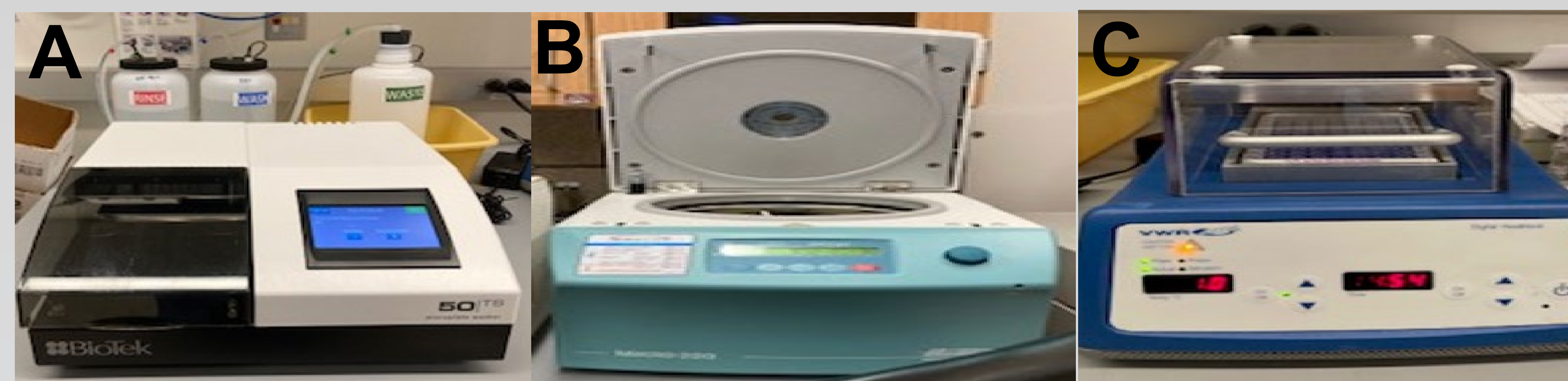
Figure 1 Essential Equipment for the Capture® Workstation. A. Semi-automated Plate Washer B. Microtiter Plate Centrifuge C. 37°C Plate Incubator
